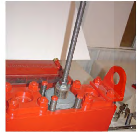
9.) Lifting the puller rod, turn the nut until firmly in contact with the washers.
