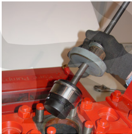
11.) Remove the puller assembly with seat attached.
