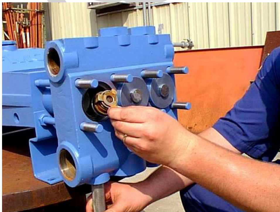
Figure 8: Removing the valve from the fluid cylinder
