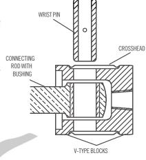
A mishap during insertion can occur causing the ruin of the pin or the
