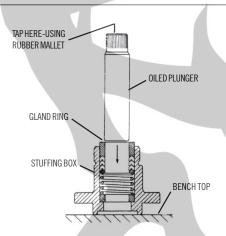
Apply oil liberally to plunger O.D. and lightly tap it through the packing. When introducing the plunger through the MA-60M stuffing boxes, also apply oil liberally to the O.D. of each extension rod to allow easy passage through the wiper box seals.
