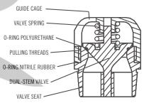
The Aurora Pump, Aplex Series valve is a precision made subassembly using threads cut into the rim of seat for use with Aurora Pump, Aplex Series setting/pulling tool. These threads do **NOT** deteriorate as proved by field experience. By locating these on the rim, setting/pulling forces are now applied only to the rim of the seat, never to the webs (or "spokes"), or to the center section. Distortion of the seat is eliminated.
