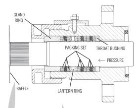
The above depicts Styles 838 and 858 packing correctly installed with all packing lips facing **TOWARD** the fluid pressure. Note that two (2) units of Styles 838 and 858 packing are positioned ahead of the lantern ring, and one (1) unit is positioned behind it. Thus lubricant entering the lantern ring is forced toward the pressure.
