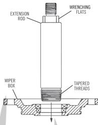
Insert the extension rod through the wiper seals with the tapered thread and entering **FIRST**. Care should be used in moving the extension rod through the seals with wrenching flats entering first. **Do not force!** The sharp corners on the wrenching flats may damage the seal lips! (Resulting in oil leakage.)
