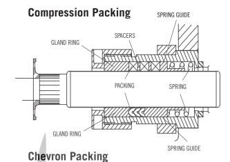
Note that the gland is screwed tightly onto the box and contacts its face. The spring is providing all of the initial compression and adjustment. No adjustment is provided by the gland.
