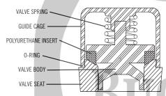
The Myers Aplex Series valve is a precision made subassembly using threads cut into the rim of seat for use with Myers Aplex Series setting/pulling tool. These threads do NOT deteriorate as proved by field experience. By locating these on the rim, setting/pulling forces are now applied only to the rim of the seat, never to the webs (or "spokes"), or to the center section. Distortion of the seat is eliminated.
