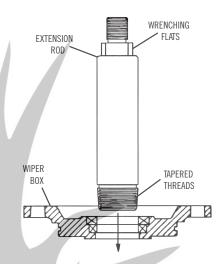
Insert the extension rod through the wiper seals with the tapered thread and entering **FIRST**. Do not move the extension rod through the seals with wrenching flats entering first. The sharp corners on the wrenching flats may damage the seal lips, resulting in oil leakage.
