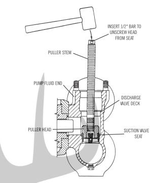
Effective pressure-sealing between tapered (male) seat and tapered (female) fluid end deck is possible **ONLY** if the tapers are absolutely clean and dry just prior to installation. Thoroughly clean surfaces using a clean solvent. Dry with a **CLEAN** shop towel.
