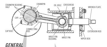
Myers Aplex Series connecting rod assemblies employ precision automotive type steel backed, babbitt-lined crankpin bearing halves which require no shims for clearance adjustment. This pump employs full circle (piston type) crossheads and hardened stainless steel extension rods, which are field replaceable.
